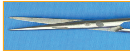
Left: Partial material attack due to acidic cement remover, and on the right due to a hemostatic agent. Cause: Excessive contact period or insufficient removal after use.
