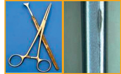
Contact corrosion: Stainless steel/Brass
