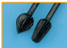
Ruts on drill bits. Cause: Reprocessing of a disposable instrument
