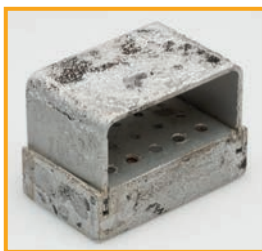
Severely attacked anodized aluminum stand
