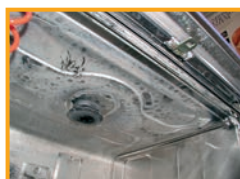
Rinsing chamber with heavy lime scale deposits
