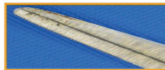
Corroded soldered seam on a carbide needle holder and carbide scissors. Cause: Phosphoric acid attack caused by overdosing the neutralization agent.
