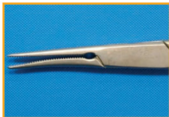
Deformation caused by improper handling
