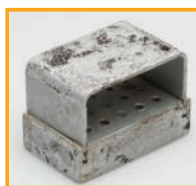
Severe material attack on the natural and color anodized aluminum surfaces of an instrument stand and containers. Cause: Overdosing of the otherwise material-compatible alkaline wash solution.
