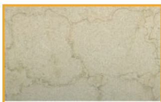
Marbling caused by impurities in steam condensate
