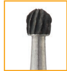
Corroded, worn out carbide drill head made of TC/CO. Cause: Application of an acid detergent.
