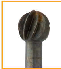
Corroded drill bit made of tool steel. Cause: Material is not suitable for machine-based cleaning without a corrosion protection layer.
