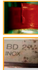
Pitting on tweezers. Cause: Over-aging of color-coding band allows harmful substances containing chloride to infiltrate.
