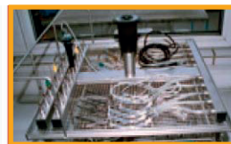
Incorrect loading of a washer/disinfector
