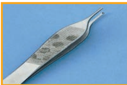
Stains on tweezers: Cause: Insufficient steam quality
