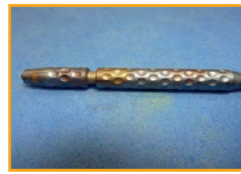
Discolored instrument handle made of titanium
