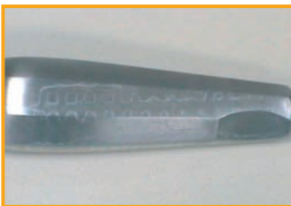
Carry-over of detergent residues due to insufficient rinsing
