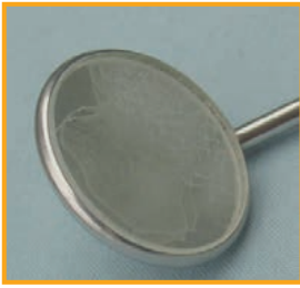
Stains caused by high salt content of rinse water
